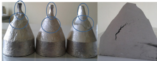
Fig. 6 Shapes and positions of internal and external shrinkage cavities
