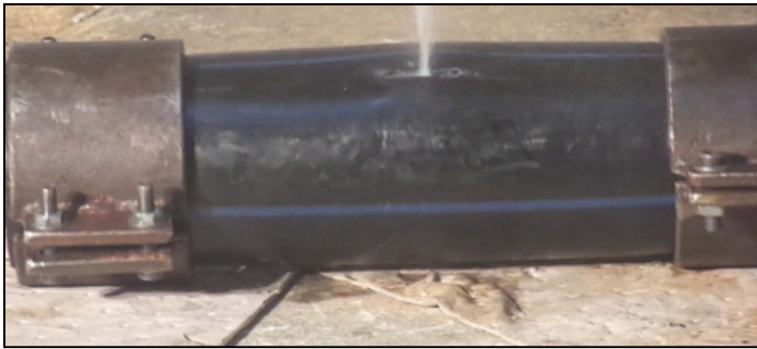
Fig. 5 Typical specimen failure of short-term burst tests
