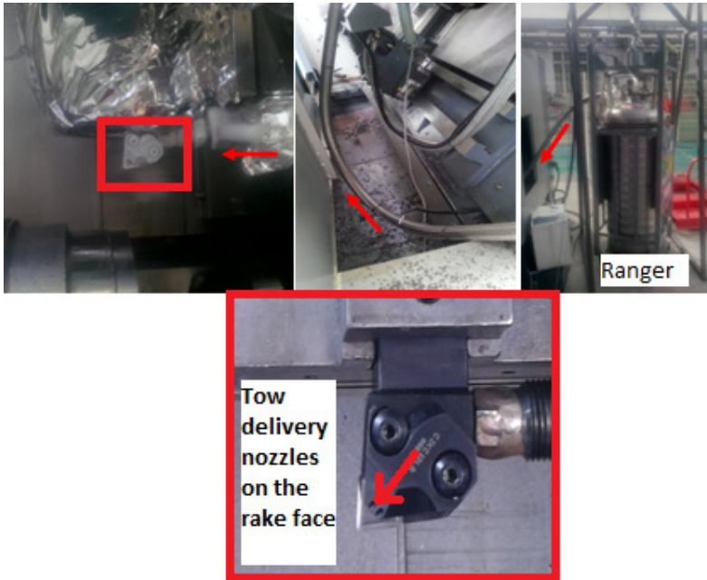
Fig. 1 Presentation of the cryogen's flow and the cutting tool
