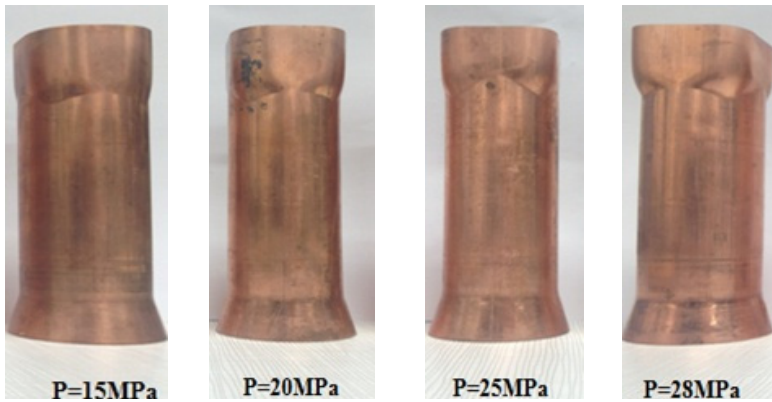
Fig. 3 Tube after hydraulic expansion with various internal pressures: experimental result
